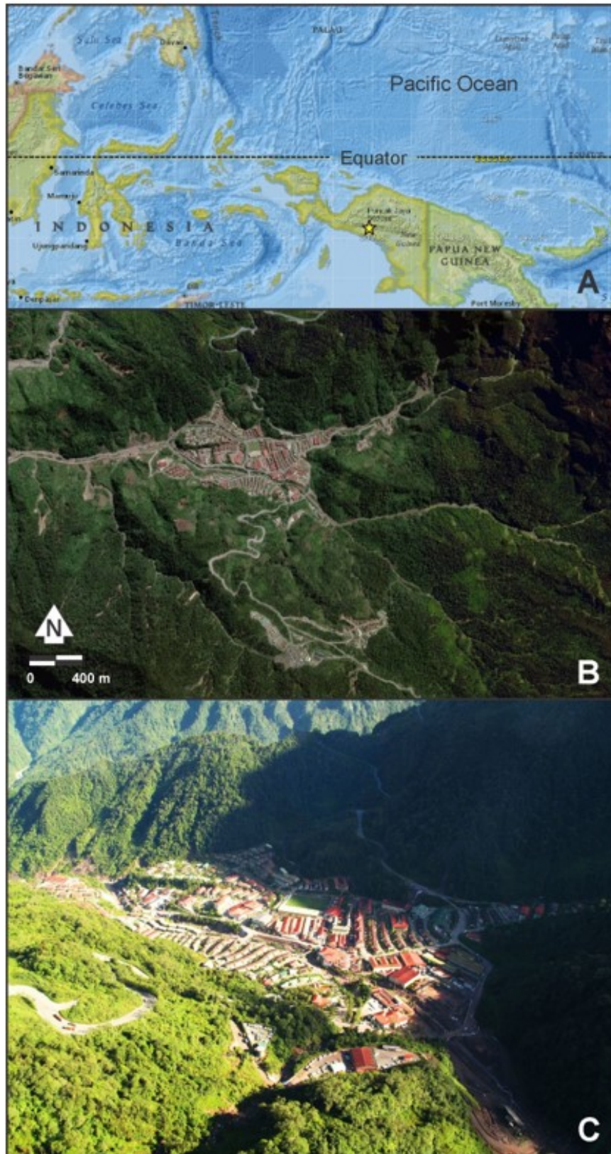
Figure 7. Tembagapura located in the province of Papua, Indonesia. (a) Regional view, yellow star indicates Tembagapura (image © ESRI and National Geographic World Map), (b) vertical image over Tembagapura showing debris flows and debris floods (image © Google Earth), (c) oblique view of Tembagapura in the steep Jayawijaya Mountains.
